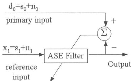
Figure 1: Model of adaptive signal enhancement filter.
